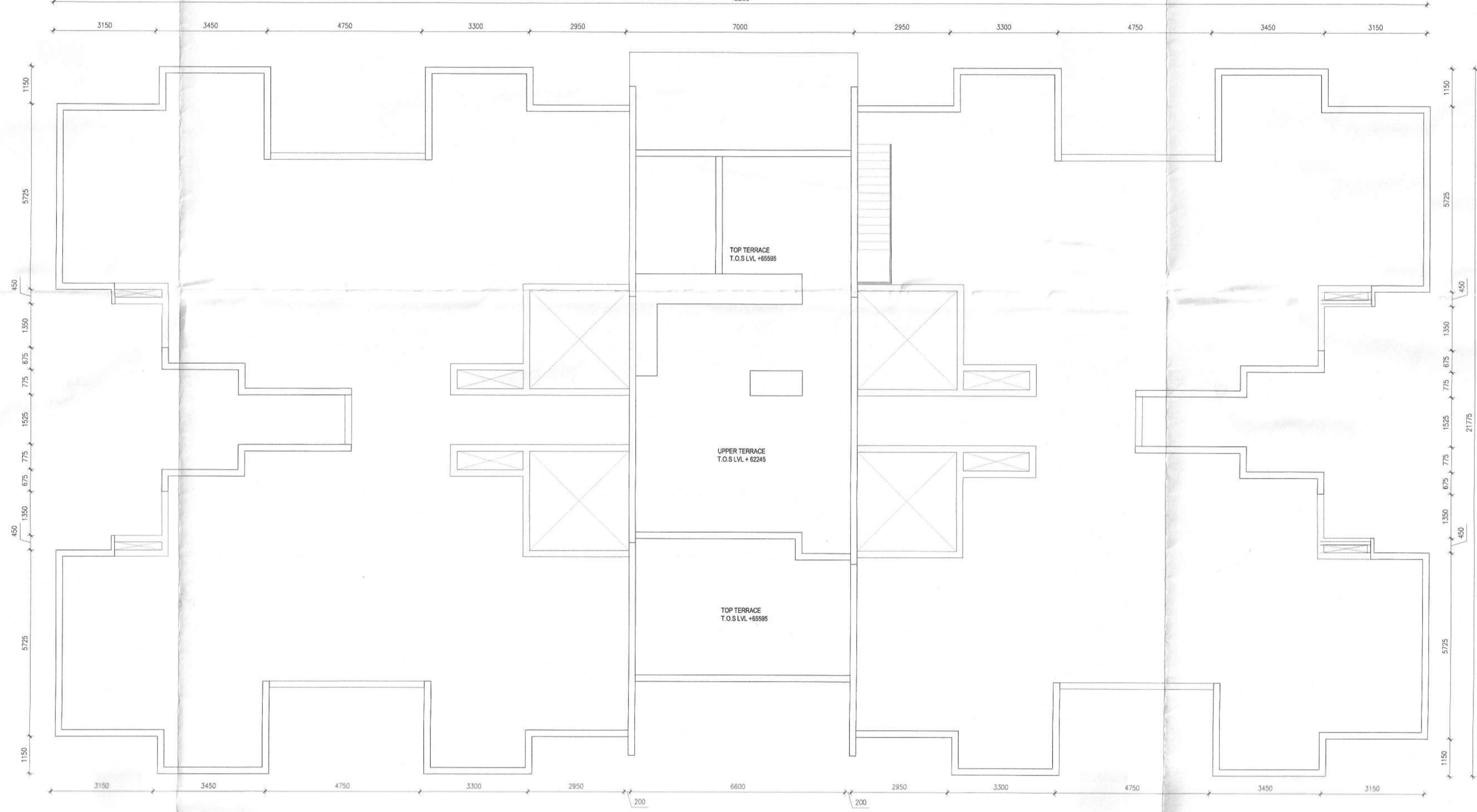
8 TOWER C2 ROOF PLAN (LVL +65595) 1:100
